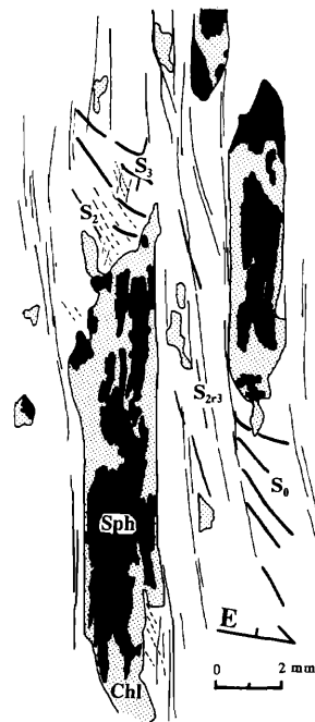
FIG. 15. Sphalerite-chlorite-quartz mineralization in low strain domains, confined between zones of intense reactivation of S_2 and S_0 . In the low strain zones, S_0 and S_2 have a less steep orientation and S_3 is preserved (see host rock at the extremities of the ore patches). It is envisaged that these sites were preferentially replaced as they microfractured and boudinaged between the zones of ductile shearing. Replacement of these sites is supported by the unclevaged nature of the mineralization and truncation of S_2 and S_3 cleavages. The ore patches are roughly zoned with a silicate rim and sphalerite core, suggesting that they are individual replacement aggregates and not elongate, transposed portions of pre- D_3 ore.
